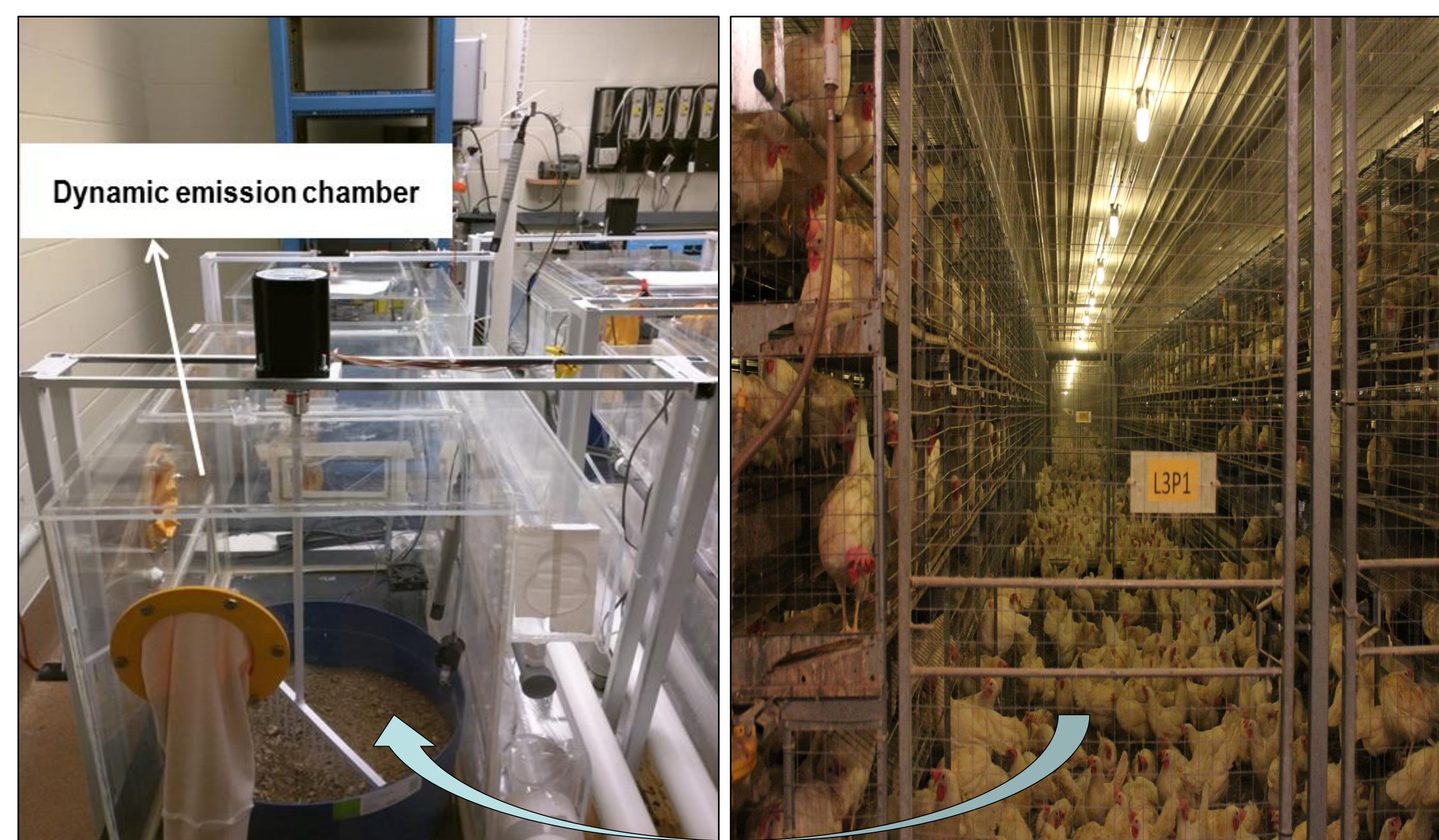
Figure 1. The acidic electrolyzed water (AEW)-spraying experimental setup
