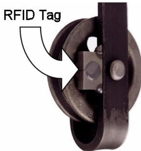
**FIGURE 9. Gambrel radio frequency identification assembly**
