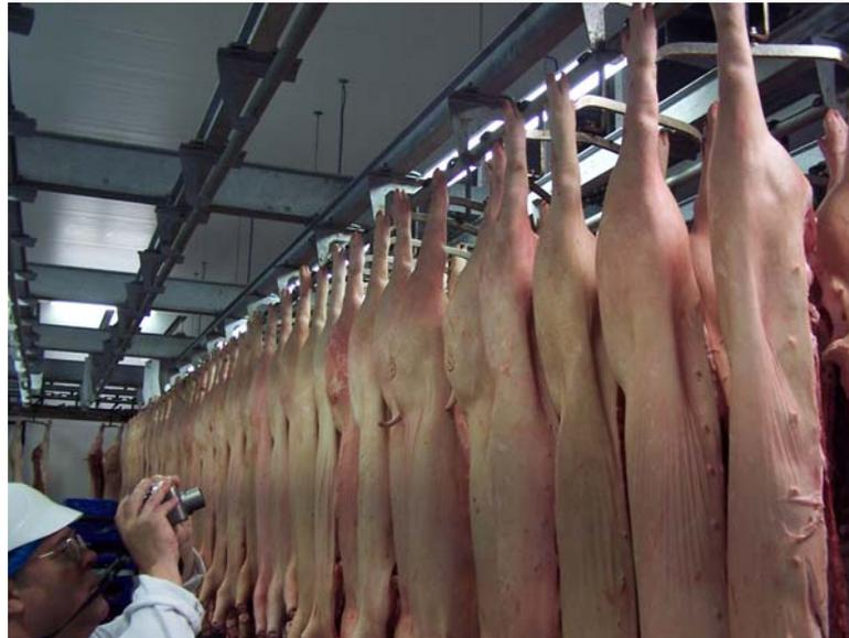
**FIGURE 11. Hog carcasses on gambrels in the cooler**
